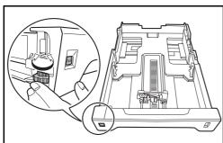
2 Turn the Paper Size Dial until the paper size you are using is visible. The paper size set here is recognized by the machine.
